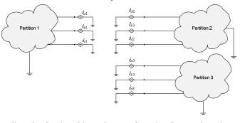
Figure 3 Creation of three subsystems from a bus disconnection point creates *six* boundary variables instead of nine.
