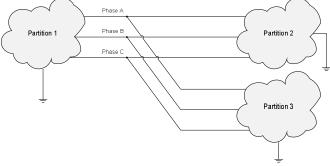
Figure 1 Tearing a bus to produce three subsystems
