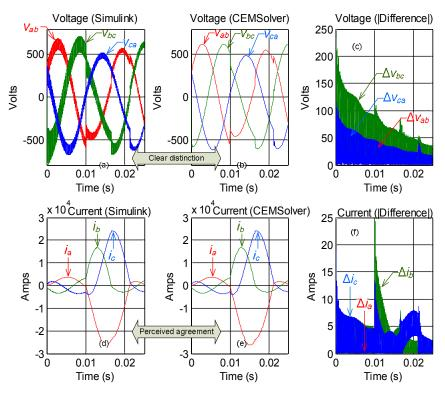
Figure 8 Node tearing: result comarison against Simulink's Tustin integration method
