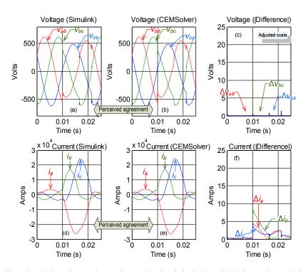
Figure 9 Node tearing: result comarison against Simulink's backward Euler integration method
