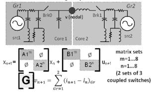
Figure 4 SSN principle showing the tearing of a node.
