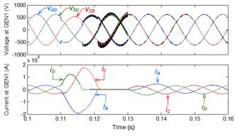
Figure 6 Accuracy comparison between *SimPowerSystems* (Tustin integration) and SSN with  $\Delta t = 50 \mu s$ .
