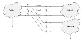
Figure 2 Addition of unknown-valued current sources at disconnection point
